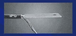
The distance between the cores and the shielding of th cable is first increased by means of the assembly tool.
